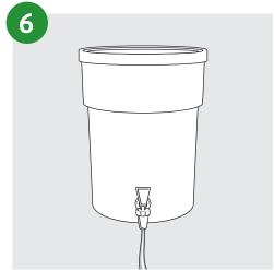
**Step 6** Drain solution from brewer through the tap outlet and allow all parts to air dry (do not dry with a towel).
