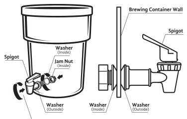
Screw the Spigot, the Inside & Outside Washers and Jam Nut together through the hole in the Brewing Container Wall
